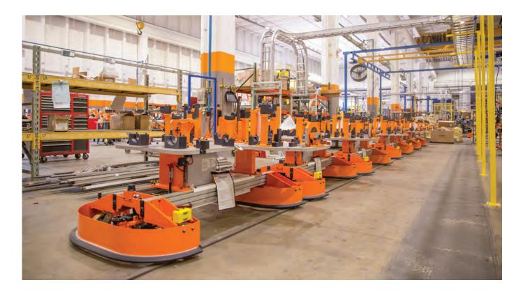
Fori Automation Inc., a specialist in automatic conveying and handling systems, relied on this flexibility while modernizing the assembly line of a large U.S. automobile plant with rail guided carts (RGCs). Each individual RGC has a safety bumper, an emergency stop switch, and optional safety scanners.
